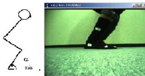
Figure 1: Markers positions of the foot and the segmentation planar model
