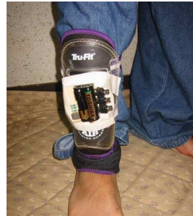
Fig. 4. "WARAJI IV" Foot motion sensing device based on acceleration sensors
