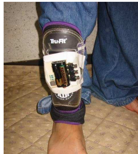
Figure 1. ”Joyfoot’s Cyber System” A new foot motion sensing device
